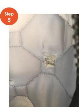
With an exacto knife cut a piece of the inner roof fabric slightly larger than the  $\frac{1}{2}$  inch hole you will need to drill to thread the solar wires from the exterior roof. Drill a  $\frac{1}{2}$  inch hole.
