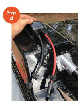
Insert the solar wires into the double entry gland leaving enough wire for the connection to the solar panel.
