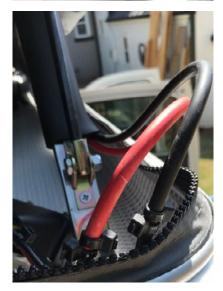
After you have finished threading, it's time to cut out a small piece of the floor fabric and drill two holes to pass the wires through the base. (Note: an alternative is to store the battery and charge controller inside the tent rather than running the wires out the bottom of the tent to your vehicle)
