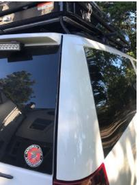
If you run all of the wiring inside the vehicle behind the panels it is recommended to add a quick disconnect behind the roof fairing where the wires enter the car. This will allow you to disconnect the solar if you decide to remove the tent at a later date.
