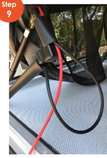
Carefully thread one wire at a time through the foam covers on the roof struts (*it can tear so be gentle*).
