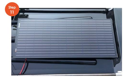
Mounting the solar cell is easier than wiring it to the vehicle. After determining the location you can set the black corner braces (from home depot) and mark the spots to drill the 3/16" holes for the rivets.
