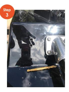
Drill two holes slightly larger than the wire through the rooftop (under the fiberglass is an aluminum plate you must drill through as well) to pass the wires.
